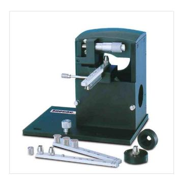
The Minidiff Plus diffuse reflectance accessory is designed for routine sampling. High performance solids analysis is made simple through the optimised zero alignment optics and Benchmark™ base-plate mounting system. Sampling versatility is maintained through the choice of either standard solids cup or Diabrase™ abrasive sampling pads. Up to 3 samples can be loaded at the same time, while the sample introduction system reduces the risk of sample spillage.
