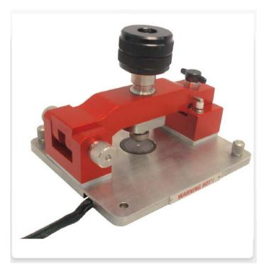
Specac's High Temperature Golden Gate<sup>™</sup> ATR Accessory is a high performance single reflection monolithic diamond ATR product offer for spectroscopic sample analysis of samples up to 300°C.
