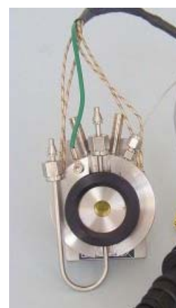
Temperature Controlled DLC version, Up to 660psi and Temperature from -80°C to 240°C
