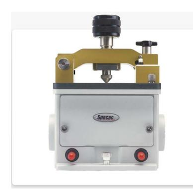
Outstanding sensitivity is achieved using high pressure contact against a solid, type IIIa diamond, selected for its unparalleled sensitivity as a single reflection ATR element together with its unique physical and chemical stability.
