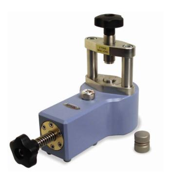
That Mini-Pellet Press is an innovative low cost solution for the pressing of 7mm KBr pellets or other small pressing applications.
